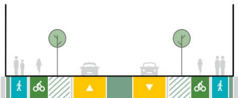
Figure 11-4: CFAF Outcome S3: Luckens Road to Brigham Creek Road Indicative 24m cross section
