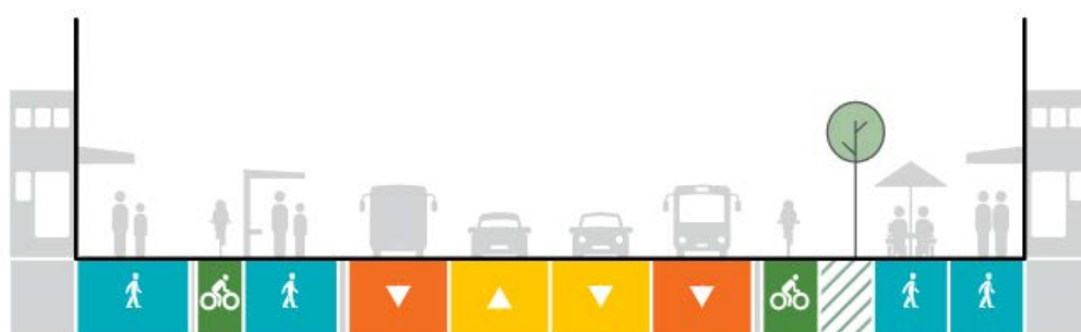
Figure 8-3: CFAF Outcome S2 (Totara Road to Tamatera Avenue) Indicative 30m cross section
