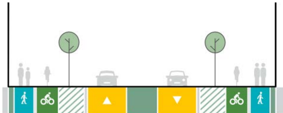
Figure 9-2: CFAF Outcome – Spedding Road East Indicative 24m cross section
