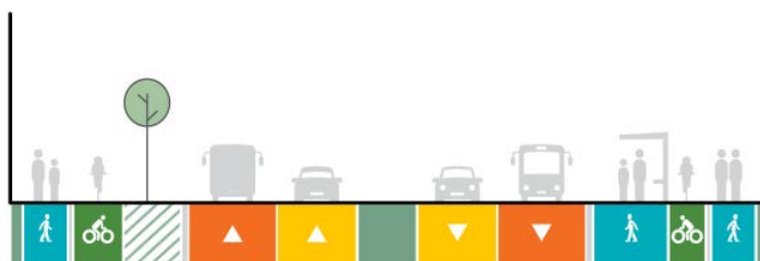
Figure 7-2: CFAF Outcome – Māmari Road Indicative 30m cross section
