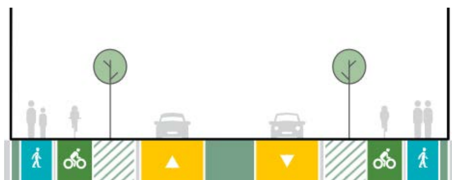
Figure 6-2: CFAF Outcome – Trig Road North indicative 24m cross section
